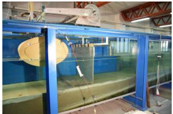
Figure 6. ShoWED in configuration 2 (rear wall at 110 cm).
