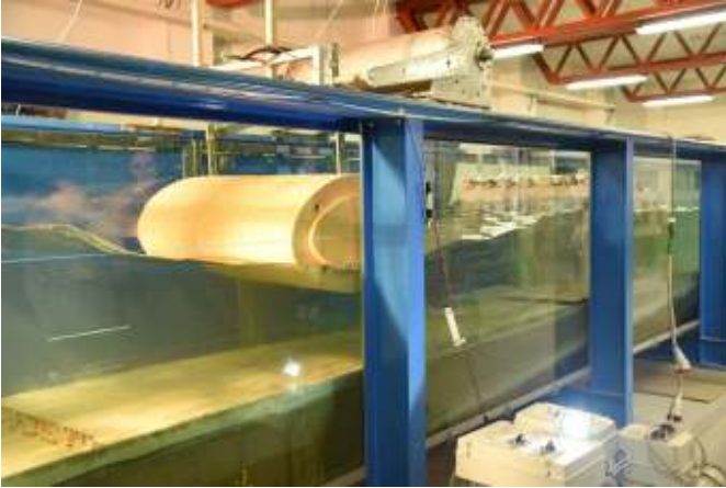
Figure 8. Floater on the trough of the wave (configuration 3, rear wall at 220 cm).
