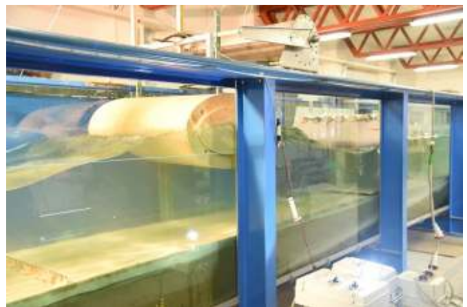
Figure 7. Floater on the crest of the wave (configuration 3, rear wall at 220 cm).
